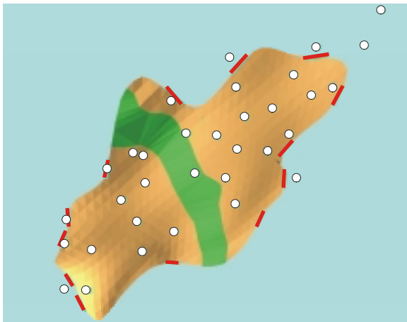
Figure 5: Geophysically constrained model of the Kelly Lake deposit showing intersections (white points) and interpreted edges (red lines). The cross cutting Olivine diabase dike is in green.
