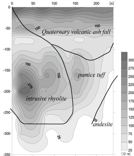
Fig.6 The reconstructed resistivity distribution by 1-D inversion computation of the SQUID data acquired over Uwamuki No.4 Cu-deposit. The SQUID data were acquired at a 10m spacing by four transmitter-loops. The orebody was placed just below the intrusive rhyolite. There is a low resistivity zone corresponding with argilic alteration.
