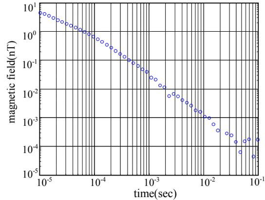
Fig.3 The magnetic field by SQUITEM over Kannondo Cu-deposit placed about 50m below the surface. The signal-to-noise ratio by the SQUID data is better than the reference coil data shown in Fig.4.
