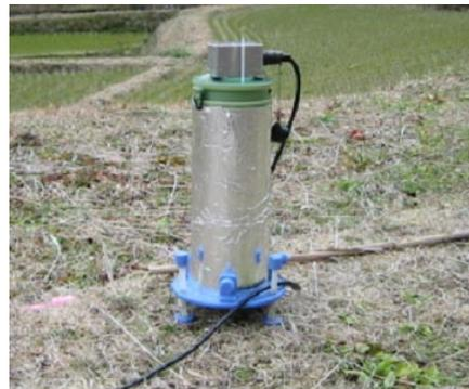
Fig.2 SQUID magnetometer for three-component simultaneous measurement. It was surrounded by aluminum foil to dull the abrupt change of the magnetic field just after current interruption in order to inject large current into the transmitter loop.
