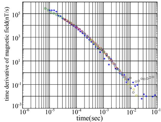
Fig.4 Comparison between the time derivative of the SQUID data in Fig.3 (\*) and the reference coil data (o). A good agreement is found between them.
