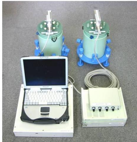
Fig.1 SQUITEM consists of three SQUID magnetometers, a PC, an A/D converter, a controller, and a battery unit.
